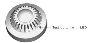
The SM-1508 detects smoke and wirelessly transmits the signal to the receiver(alarm control panel). It also has a built-in buzzer to warn people in the immediate vicinity. For testing purposes the detector is equipped with a testing button. The detector makes regular auto testing and reports tis condition to the system regularly for full supervision. The LED indicator can be turn on / off upon your requirements.
